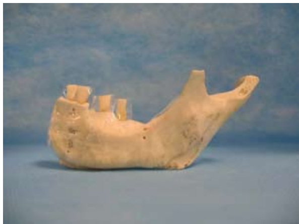
Figure 3. The test teeth were mounted in a dry sagittally-sectioned mandible and CBCT scans and periapical radiographs were made
